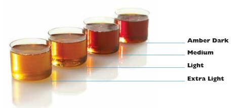
Syrups are classified by determining how much light passes through the maple syrup. The transmission of light is measured using optics. a spectrophotometer is used for this analysis technique.
